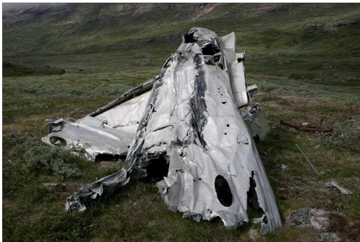
Figure 10. The aft part of the 13013. The oval-shaped window just above the tear, combined with the 14-cylinder radial engines, provided the first clues determining the aircraft type.
