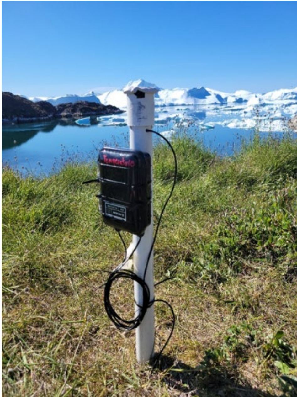
Figure 24. Air and surface soil temperature datalogger at site 1-03. Photo: C. Bonsell, 2024
