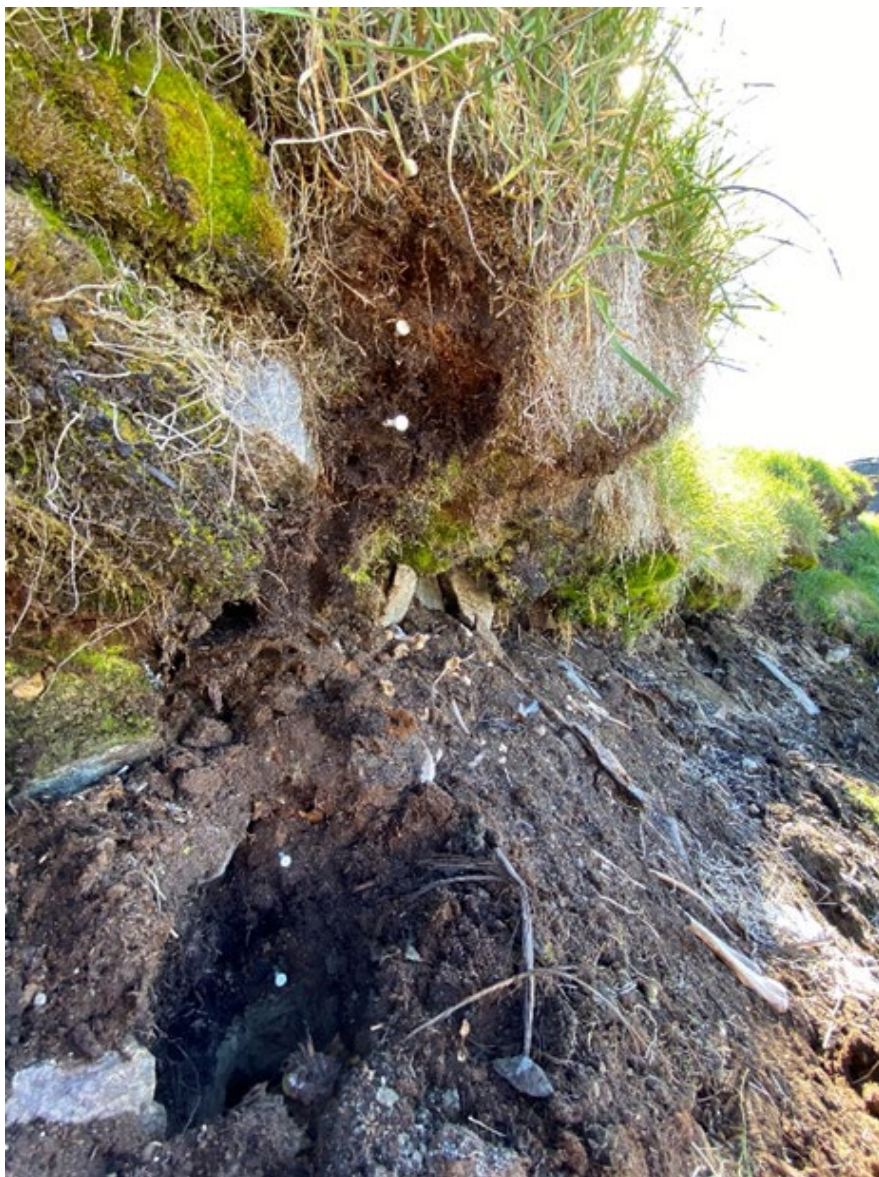
Figure 21. A soil profile exposed along the bluff face, with white markers indicating transition zones. Photo: C. Benton, 2024.
