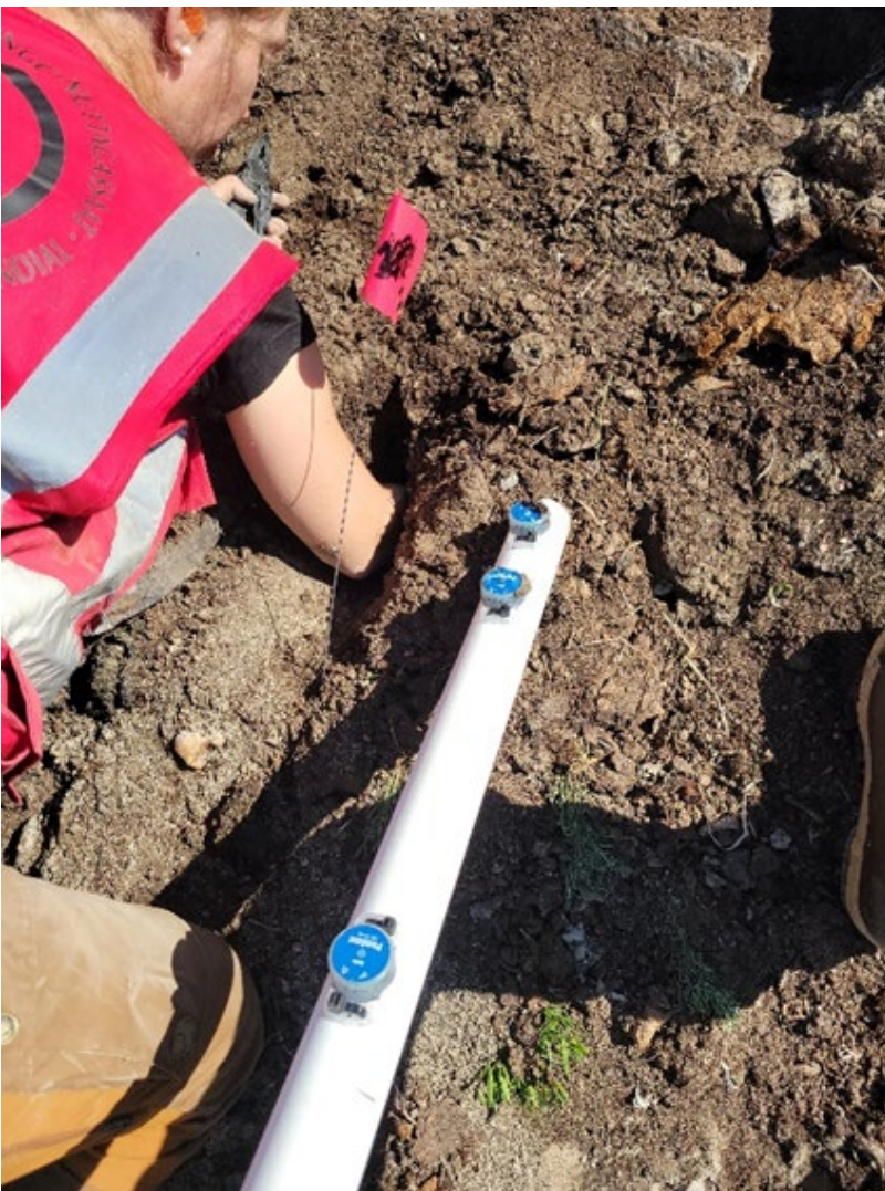
Figure 23. Soil temperature datalogger array showing three different dataloggers set to be installed at different depths. Photo: C. Bonsell, 2024.
