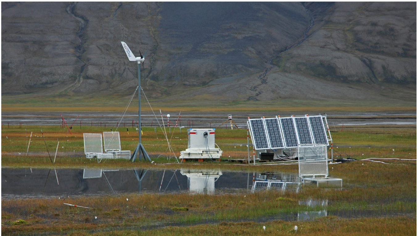
Field instrumentation in Adventdalen, Svalbard, Norway, to measure greenhouse gas emissions in tundra bogs that are underlain by permafrost (Andrea Schneider).
