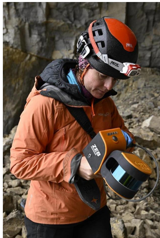
Figure 11: Gabriella Koltai surveys WUL-8 using the LiDAR ZEB Horizon, GeoSLAM. The Cardo Outdoor communication device can be seen on the helmet.
