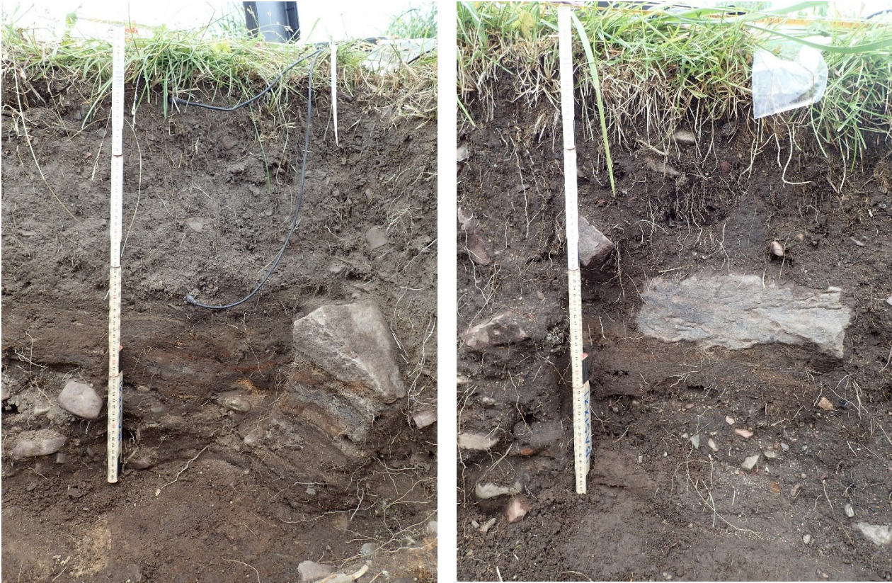
Figure 16. North profile at x 0.0/y 2.5 (left) and East profile at x 0.7/y 3.0 (right) where measurements and samples were taken. The Tinytag sensor were moved from the North to the East profile to avoid the backfill from 2019.
