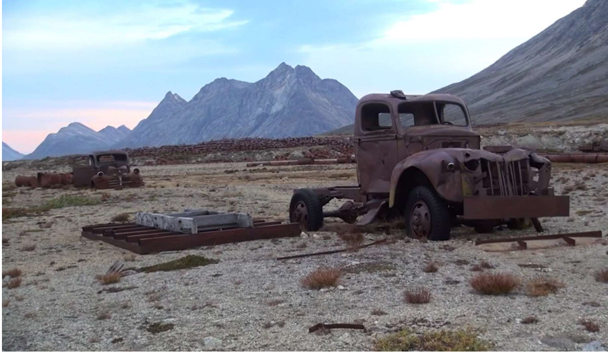
This is Dodge pickup #1 visible to the left and Marmon-Herrington Ford 4x4 #2 at the right. This truck has a reinforcing strut through the front fender possibly for snow removal equipment but does not show signs of the headlights being set up for that. Photographer unknown.
