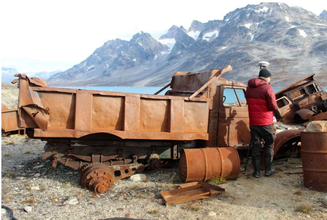
(dump body #8 at the extreme left) This is Sterling #11 and Sterling #7 at the far right. The cast vee radius rod (arm) and rear suspension typical to the HC145 model is quite apparent in this view (Sterling #11).
