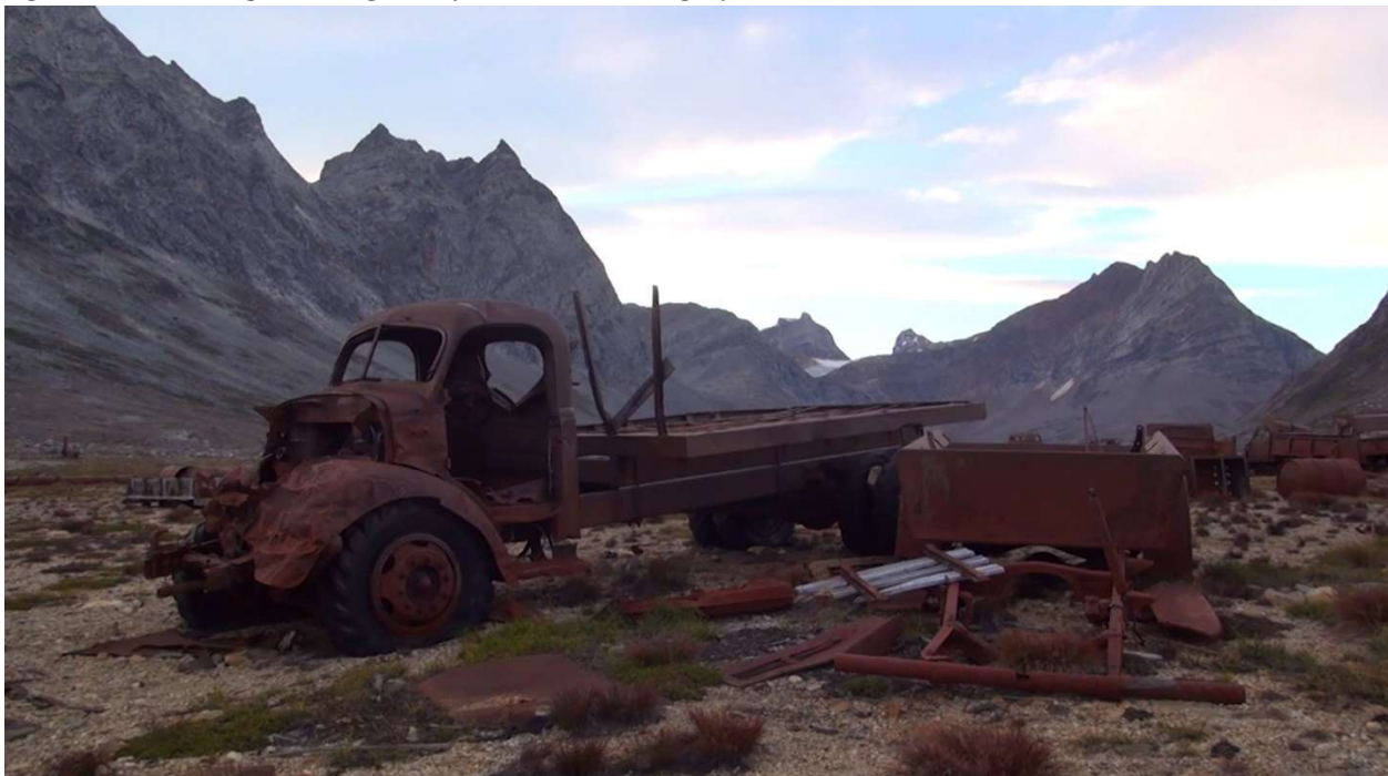
This is Dodge pickup #1 visible to the left and Marmon-Herrington Ford 4x4 #2 at the right. This truck has a reinforcing strut through the front fender possibly for snow removal equipment but does not show signs of the headlights being set up for that. Photographer unknown.
