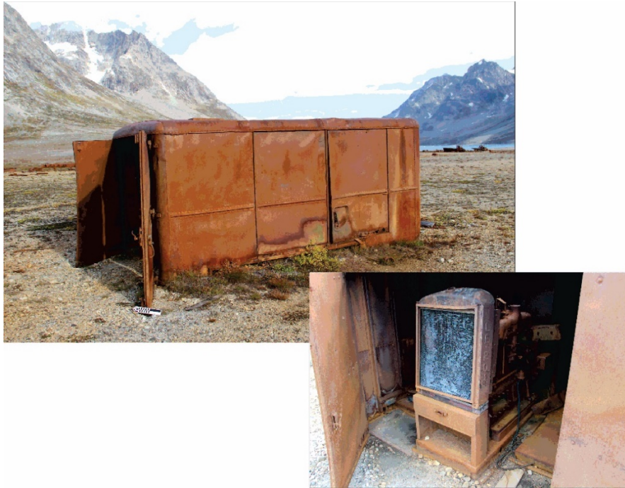
Fig. 19. A LeRoi engine, gas powered generator stationed next to the hangar inside a protective steel Enclosure at BE-2 (photos: H. Lange 2018).
