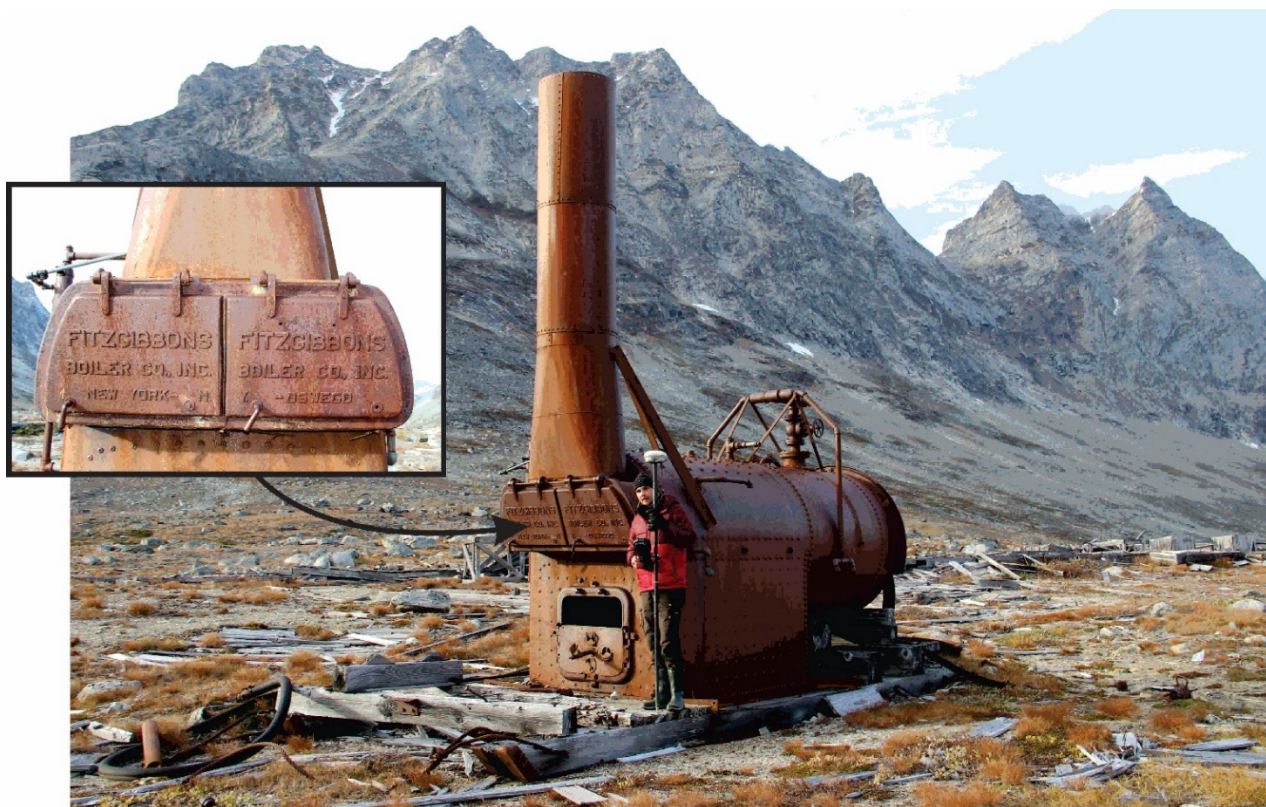
Fig. 55. A lonely boiler far from home. This industrial boiler was manufactured by the FitzGibbons Boiler Company, Inc., Oswego, New York. Harmsen shown collecting dGPS point (photo: H. Lange 2018).
