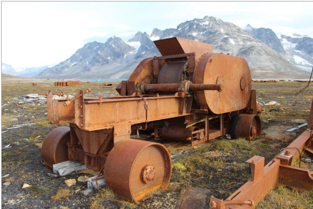
Fig. 54. Rock crusher used to produce gravel for the airstrip at BE-2 (photo: H. Lange 2018).
