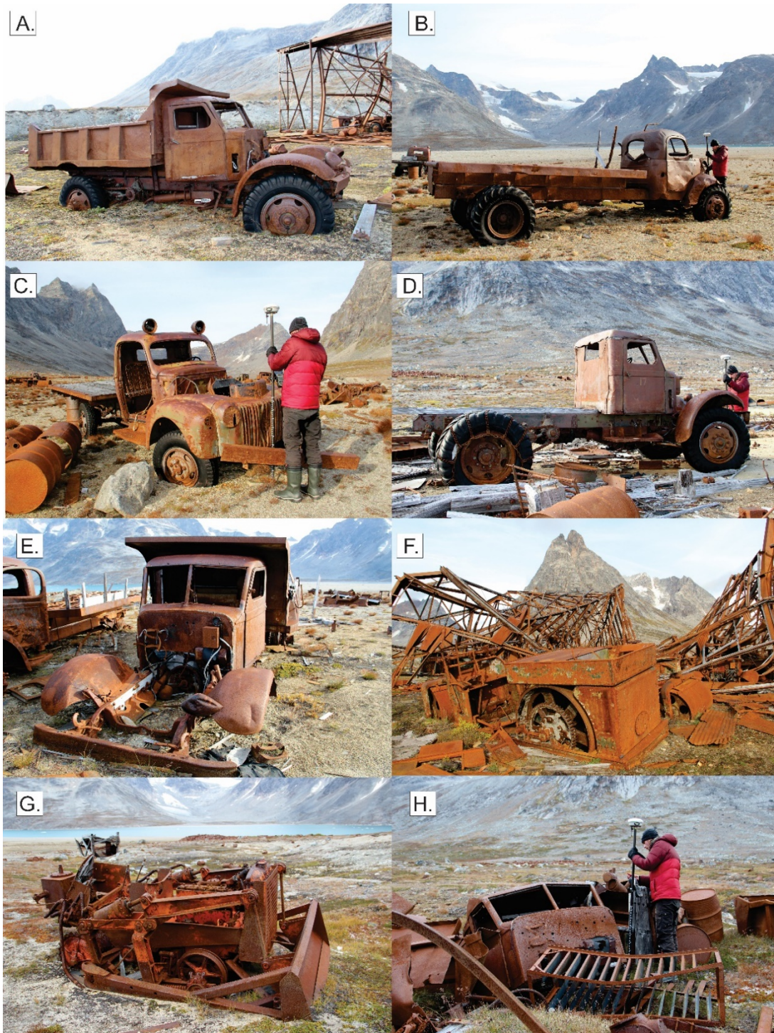
Fig. 39. Examples of derelict vehicles observed at BE-2 in September 2018. (A) Vehicle no. 8, Sterling HC 145 truck, ca.1940-41. 6-cylinder, gasoline SRKR Waukesha engine, 9 to 10-ton payload., (B) Vehicle no. 12, 23. Reo Model 23 or 25. 2 1/2-ton 6x6 truck, also known by the nickname 'deuce and a half', or just 'deuce.' This model was designed as a tactical cargo truck for the US Armed Forces. Load-rated (2,300 kg; 5,000 lb) could operate off-road in all weather; (C) Vehicle no. 23, Reo Model 23 or 25; (D) Vehicle no. 24, Sterling HC 145 truck with snow chains still present on the rear tires.; (E) Vehicle no. 11, Sterling MC 96, similar to HC 145 built with 60-inch wide cabs vs. the HC145 64-inch wide cab; (F) Vehicle no. 1, road roller, unknown make and model; (G) Vehicle no. 25, possibly Catepillar; (H) Vehicle no. 26, unidentified cab, no engine or chassis.
