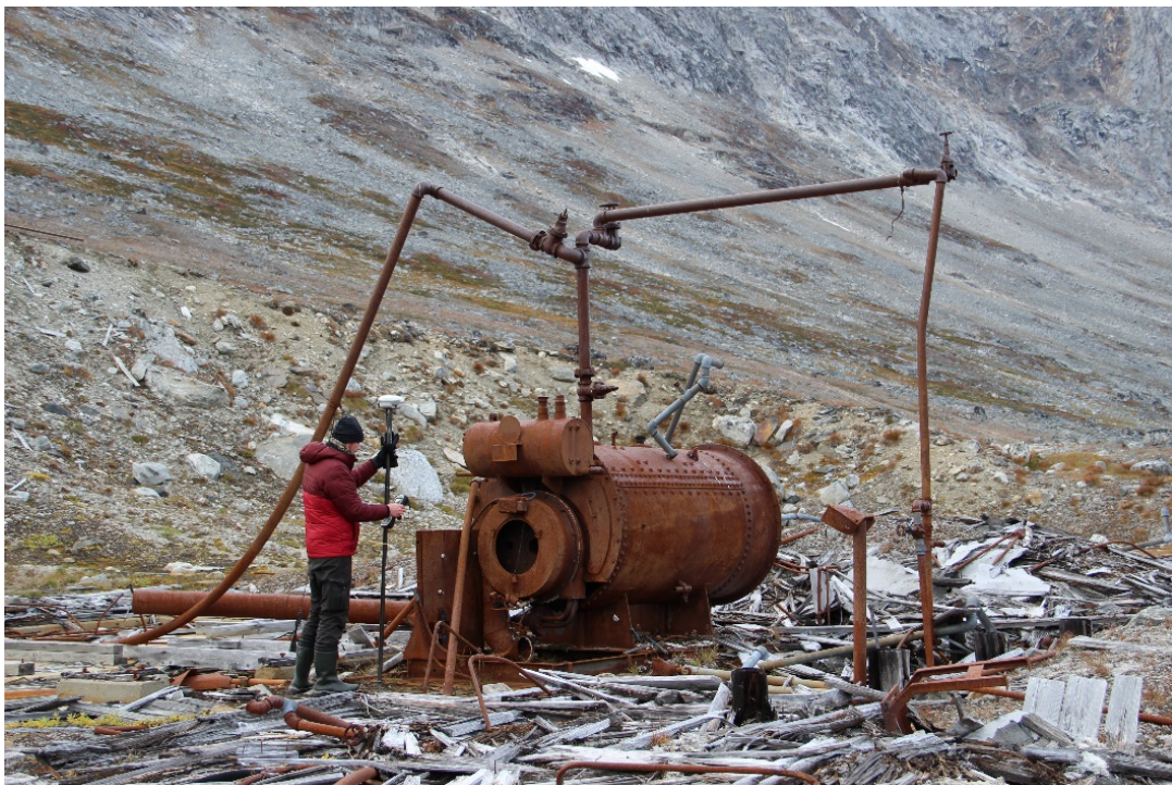
Fig. 17. A large pump was observed near the well in the northwest part of the camp of BE-2. This large industrial pump would have transported water throughout the base (photo: H. Lange 2018).
