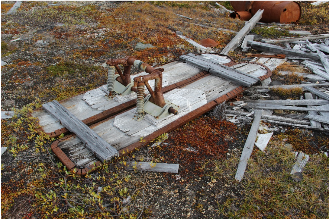
Fig. 51. Modified snow skis, possibly attached to a trailer pulled by the M-7 (photo: H. Lange 2018).
