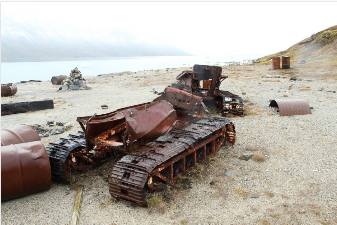
Fig. 41. Remains of an Allis-Chalmers M-7 Snow Tractors (Vehicle nos. 31-32). These small half-track vehicles were used for rescue operations in remote and snowy terrain and are extremely rare WW2 relics (photo: H. Lange 2018).
