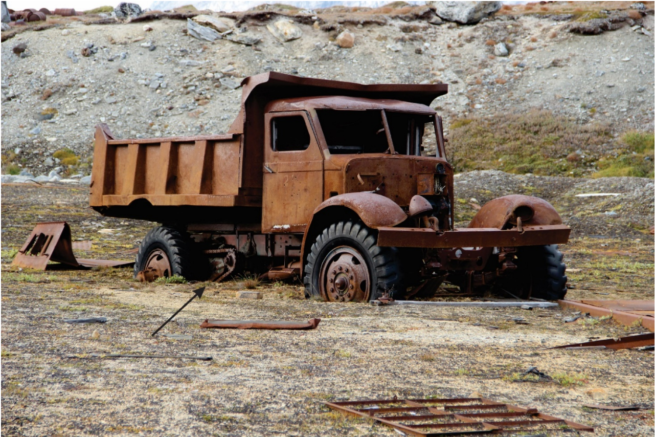
Fig. 29. A lonely Sterling HC 145 truck lying derelict at BE-2. Note arrow pointing to the rear axle chain-drive system. Chain-drives assisted navigating difficult terrain and pulling heavy pay-loads at BE-2 (photo: H. Lange 2018).
