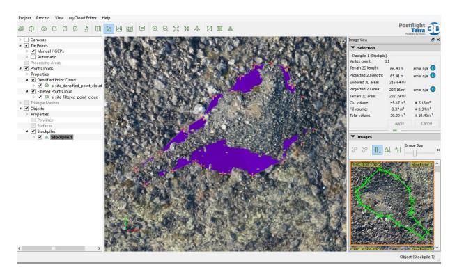
Figure 65: Screenshot of software stockpile calculation window. After definition of pile (smaller right hand window) the program calculates volume. Mikkel Myrup *del*.
