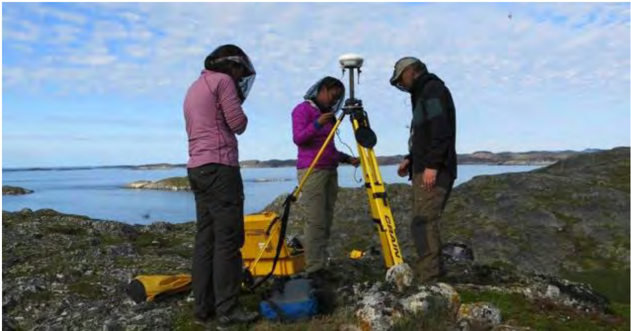
Fig. 6 Setting up the DGPS base station. Photo: Pauline Knudsen
