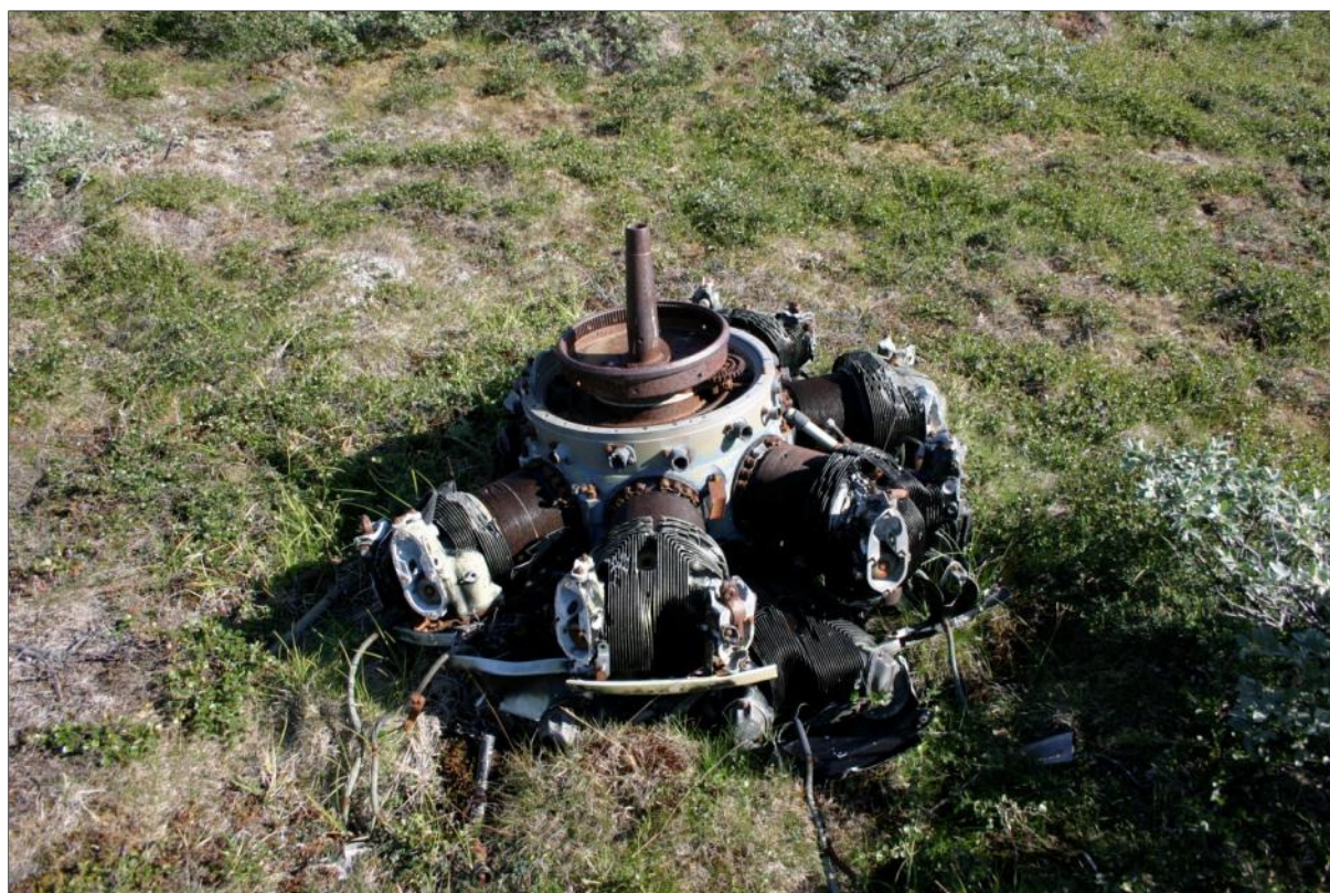
Figure 11. One of the two radial 14-cylinder Wright Cyclone 2600s.
