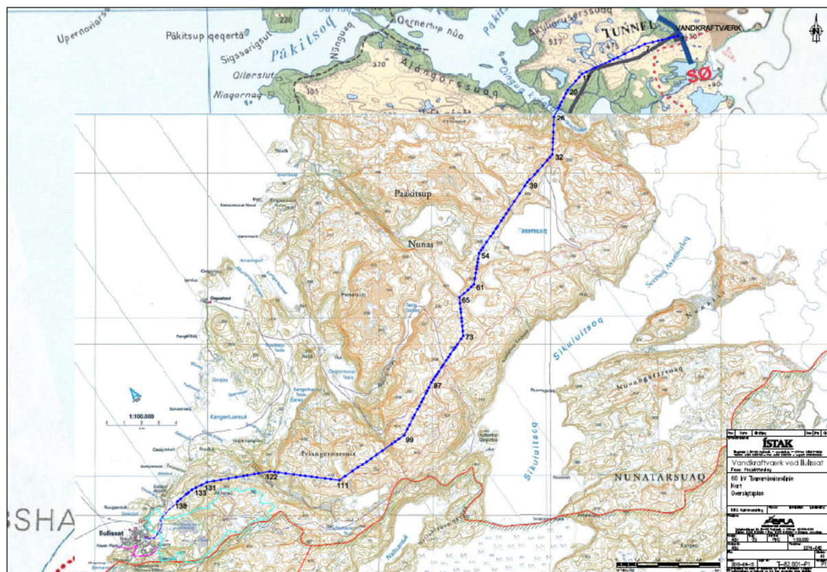
Map 1. This map made by ÍSTAK shows the transmission line and the position of the masts. A list of mast coordinates were also handed out to the NKA.
